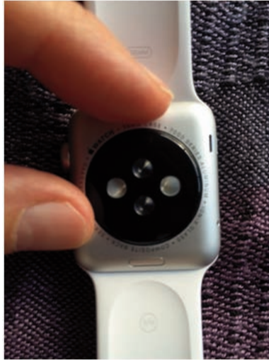
The back of the Apple Watch has four sensors, which include infrared and visible-light LEDs, in addition to photosensors.
